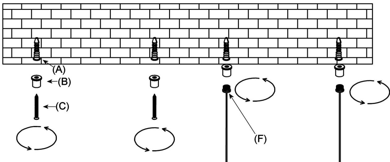
Using the fixing positions marked on your ceiling drill fixing holes taking care to avoid electrical supply cables. The unit is supplied with general purpose hardware for fitting the metal ceiling fittings (B) to a sound ceiling surface. Many situations require more specialist fittings, if you are in any doubt we recommend that you seek professional advice. The light should be fixed to a ceiling, joist or batten suitable to support the weight of the light fitting.
